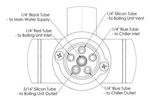
2. Position boiling water unit underneath the sink directly beneath the tap head. Observe attached labels (ensure when pipes are cut to de burr ends before fitting).
